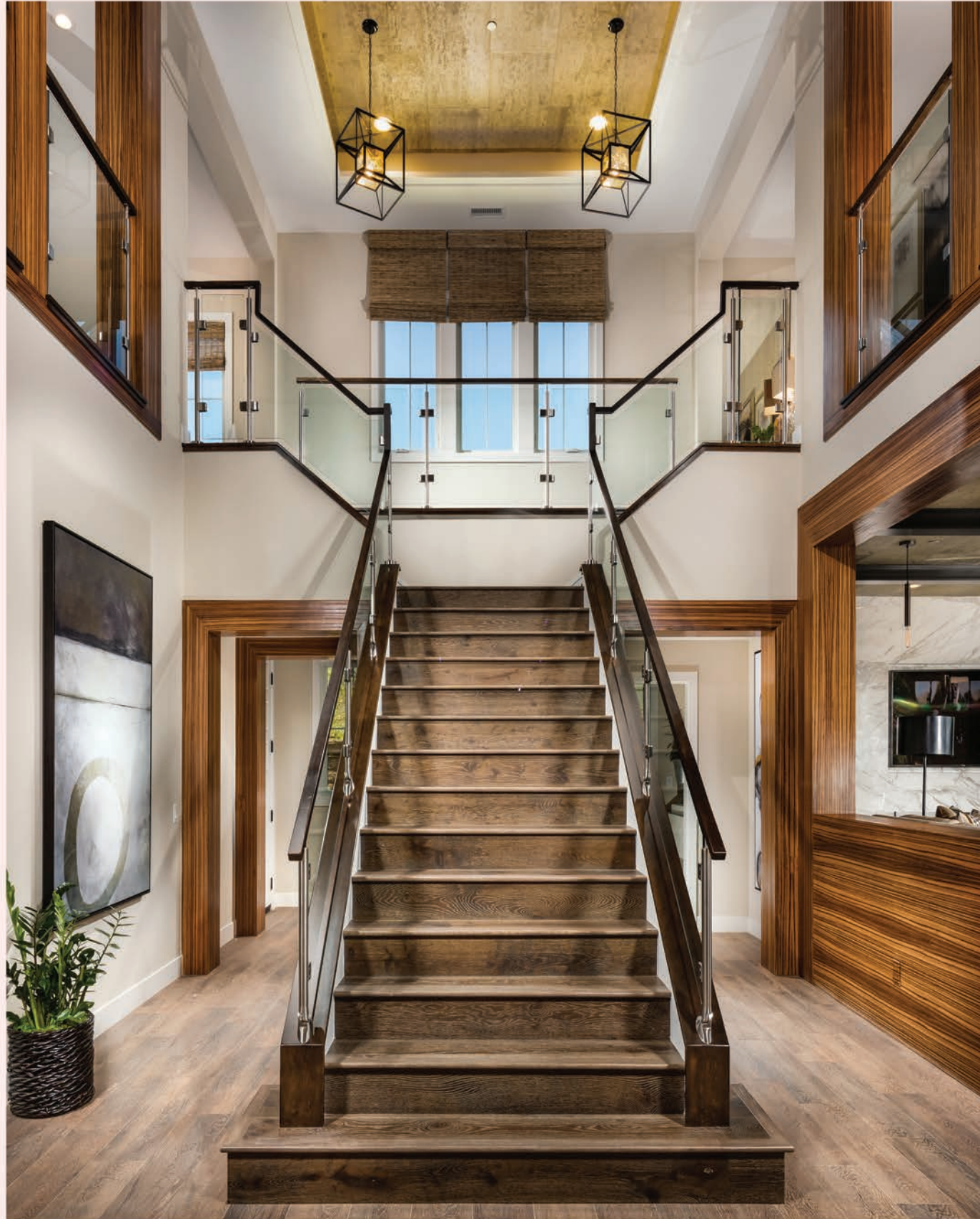
Custom Post Handrail System with SentryGlas® Laminated Glass
