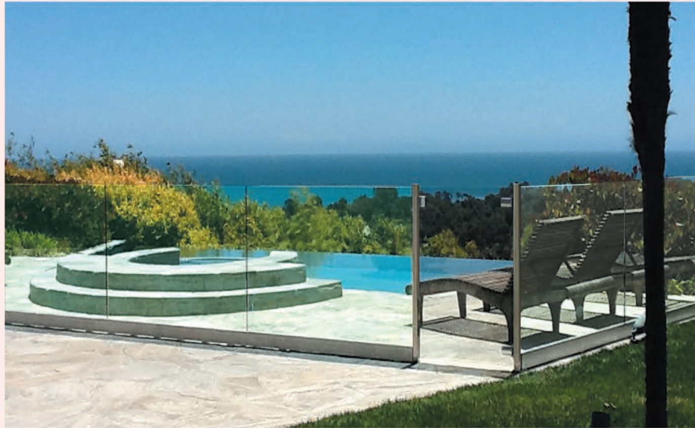
Brushed Stainless Steel Rapid Guardrail System with Laminated SentryGlas®
