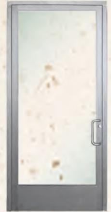
NARROW 2" vertical stile, 2", 3 1/4", 5 1/8", 10" or custom height top/bottom rails
