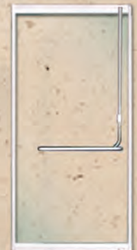
FF Style Door w/ PL100 Panic Device/ A exterior handle
