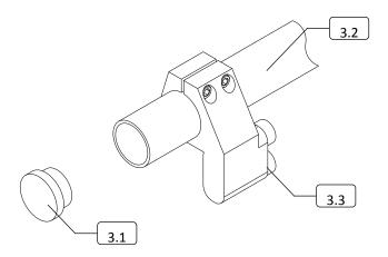
Insert 3.3 stop in 3.2 tube ( do not tighten yet )
